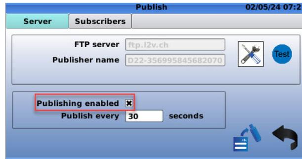
The "FTP server" field is then automatically filled with the FTP server set in the device. The FTP server access settings can be changed by pressing the
