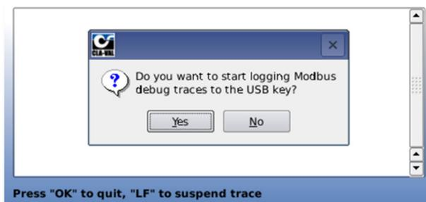
If the debugging tab is closed, then a pop-up message will appear which asks if the logging on the USB key should continue.
