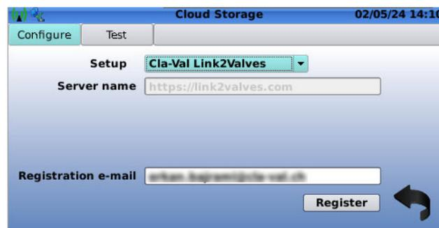
To connect to the CLA-VAL web server and view data on Link2Valves.com, select the Cla-Val Link2Valves option. Then, register using your email address. For more details, refer to Chapter 4.3.3 (insert link).
