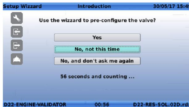
Selecting "**No, not this time**" will exit the "**Setup Wizzard**", but the latter will be launched again automatically after the next unit reboot.
