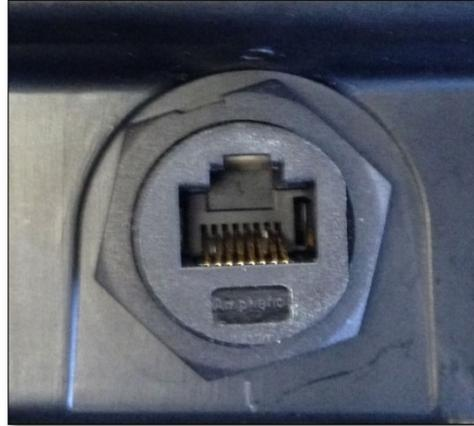
In the Ethernet port, it is possible to connect RJ-45 Ethernet cables, just like those shown in the photo on the left side.
