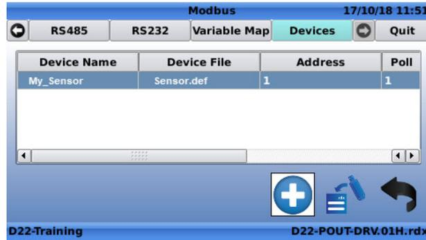
g. These inputs/outputs will can be configured as a normal input/output. Example of a specific D22 sensor interface definition file.
