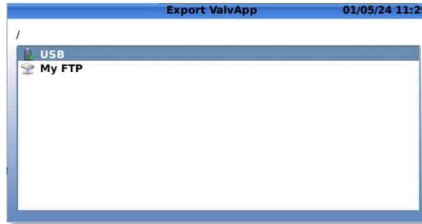
The USB option gives the possibility to export the application to the directory of the connected USB stick, the FTP option enables the user to export the application to an FTP server.
