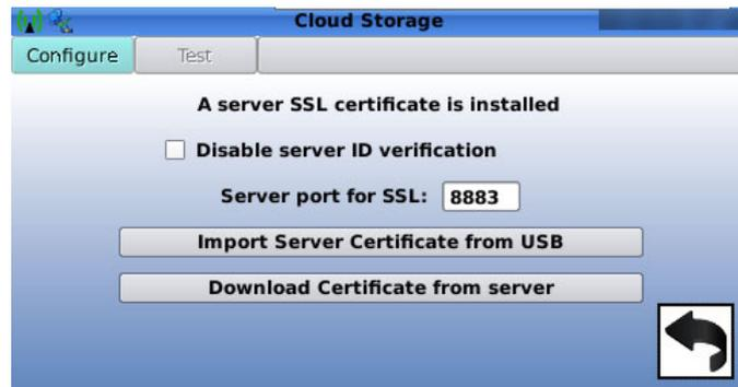
The screenshot shows the 'SSL Options' configuration window. It displays the message 'A server SSL certificate is installed'. There is a checkbox for 'Disable server ID verification' which is currently unchecked. The 'Server port for SSL' is set to '8883'. There are two buttons: 'Import Server Certificate from USB' and 'Download Certificate from server'.
