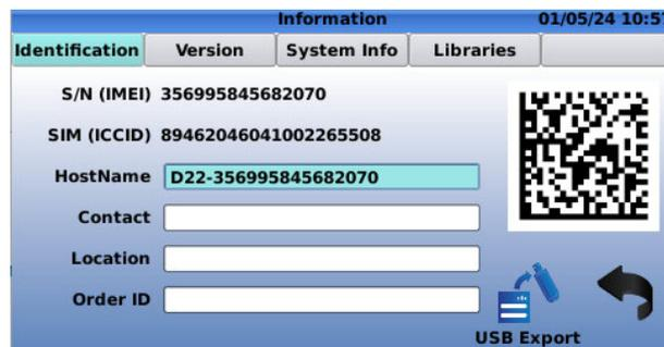
Device identification information with "**S/N (IMEI)**" the serial number of the device, and "**SIM (ICCID)**" the SIM card identification number.
