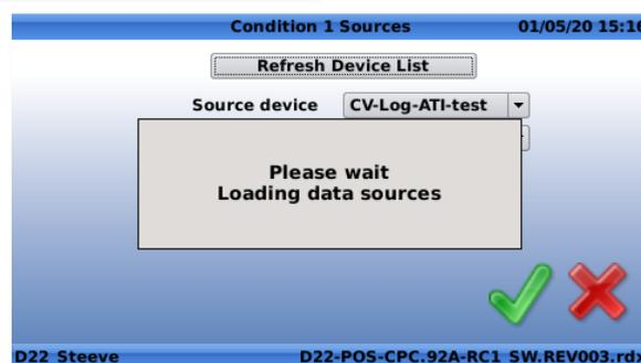
5. It is now possible to select the "**Source device**", that will be the desired CV-Log. When selected, click "**OK**", that will update the list of the channel available for the selected CV-Log.
