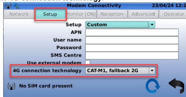
**4G connection technology:** Offers the possibility to choose between numerous options of communication depending on the coverage constraints, and the geographical situation of the device.
