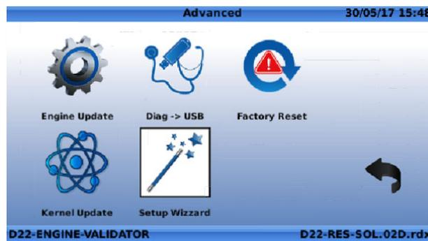
When the "**Setup Wizzard**" is launched, the user has 1 minute to react before it deactivates and the unit gets back to normal use.
