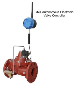
CLA-VAL SERIES D35 switches a latching solenoid by means of a CLA-VAL D35 autonomous electronic valve controller, according to predefined time, flow, level and/or pressure rules, or upon remote command.
